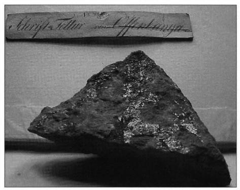
Figure 4. Sample of "Schreib Tellur" or "graphic tellurium" (sylvanite, AuTe<sub>2</sub>), so named because of the long pencil-like rods. Sylvanite was almost certainly the mineral from which Müller von Reichenstein isolated tellurium. This superb 15-cm diameter sample was collected and labeled by some unknown collector as long as 200 years ago. The collection site was Offenbanya, now known as Baia de Arieş.
